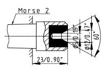
A0166030A-Z Blunt full centre long dia.48mm (1.890") for internal holding fixture MT2
