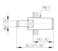
A5560012A-Z Impregnated diamond for grinding wheel grit 120-320 with fitting taper MT1 shortened (clamping length 19mm (0.748"))
