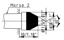
A0138004A-Z Full centre A long dia.20mm (0.787") for internal holding fixture MT2
