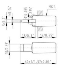
A2813077A-Z Single point diamond 0.1 carat, with fitting taper MT1 shortened (clamping length 19mm (0.748"))
